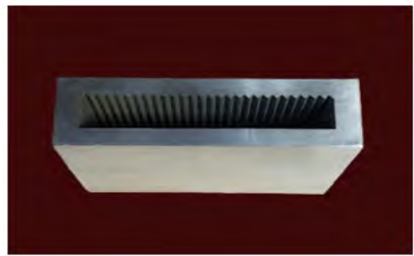
Figure 1: Carbon steel alloy dies used to fabricate samples in the study
