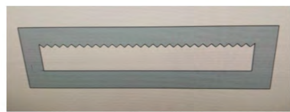
Figure 2: Ridges incorporated in the design of the dies
